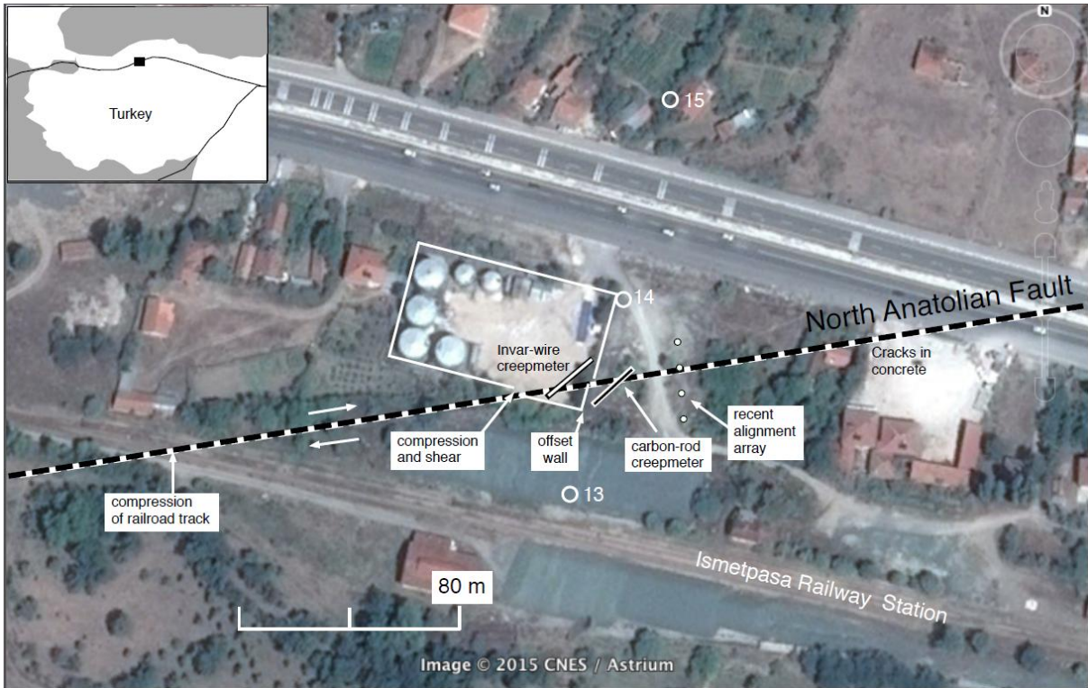
Figure 1. Google Earth view of the Isetpasa maintenance yard showing the North Anatolian Fault and locations of invar and carbon-fiber creep-meter (40.8698°N, 32.6250°E) and nearby geodetic alignment array points 13-15 (Aytun, 1984), and the eastern wall of the maintenance yard, cross the fault at 66°. The railroad crosses the fault at 24° in compression and has required occasional re-alignment and shortening to accommodate creep.
