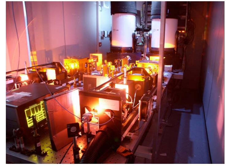
The PSC observations at Rothera and South Pole were made with the UIUC Fe Boltzmann/Rayleigh lidar, which is a dual-channel resonance-fluorescence lidar operating at 372 and 374 nm with full-diurnal coverage.
