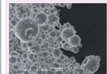
Scanning electron microscopy (SEM) image of pure siRNA particles formed at 50 °C from a 10% aqueous solution.
