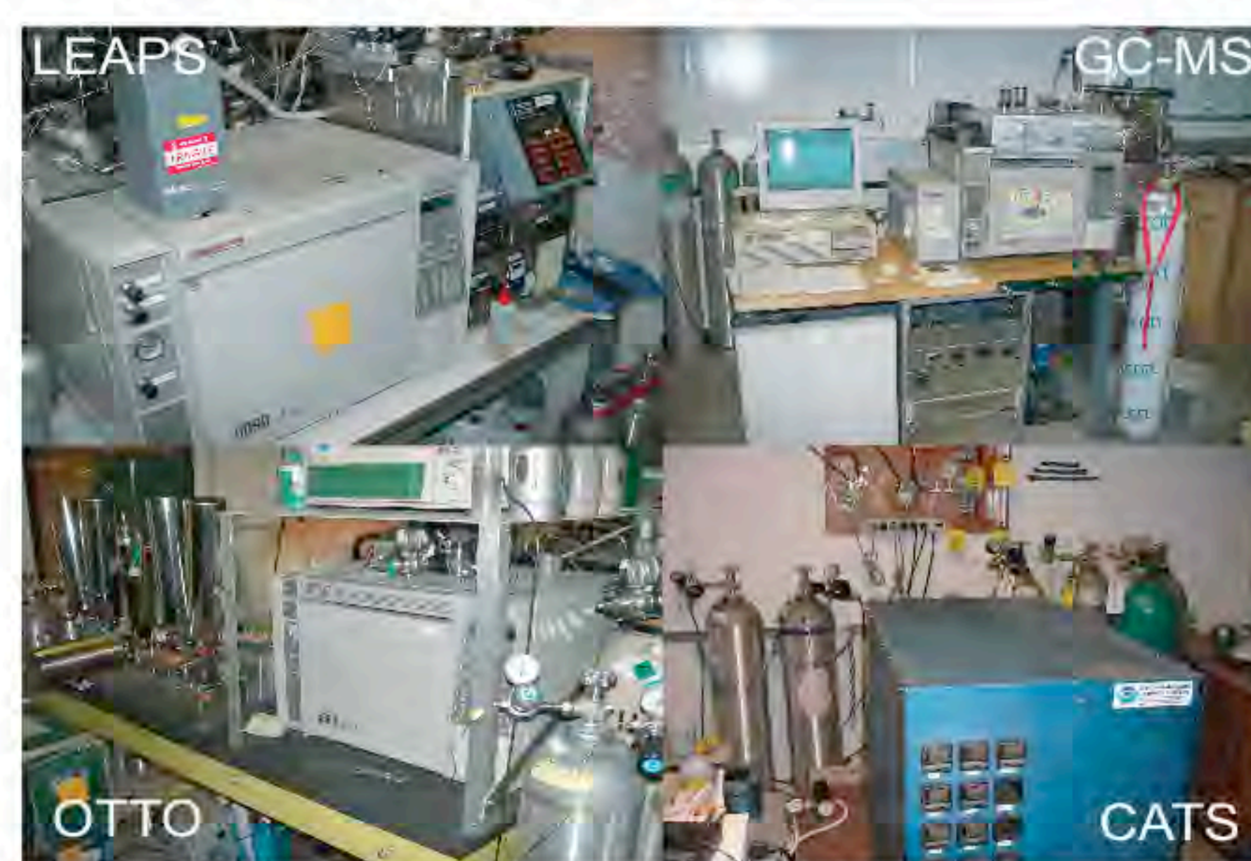
Fig. 3 Current NOAA/ESRL GC systems, Low Electrophilic Attachment Potential (LEAPS), GC-MS, and OTTO for analysis of flask samples in Boulder, Colorado (ESRL), and the in situ Chromatograph for Atmospheric Trace Species (CATS) at five baseline observatories (Mauna Loa GC pictured here).
