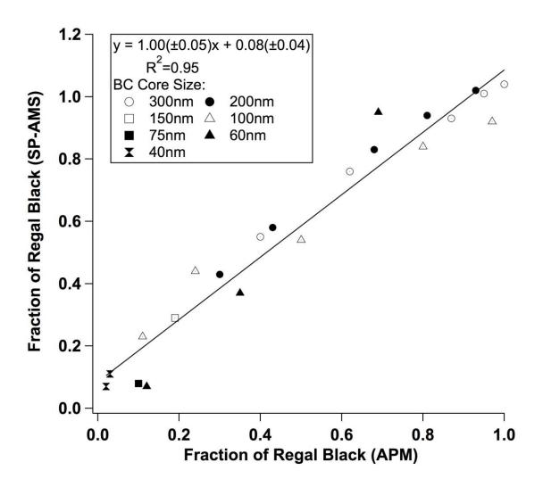
Taking into account changing RIE for rBC and BES as the particle beam becomes narrower. SP-AMS can provide an accurate quantification of rBC down to 5% by mass for internally mixed particles.
