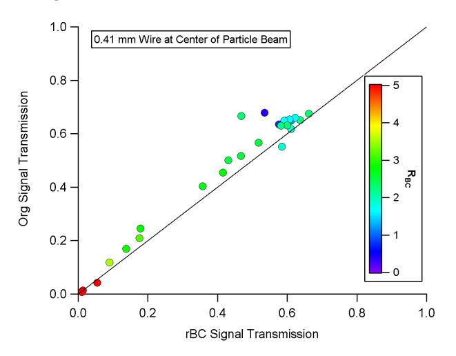
Org and rBC signal transmissions decrease together with increasing DOS coating and narrowing of particle beam, suggesting that the effective particle beam widths for rBC and DOS are similar
