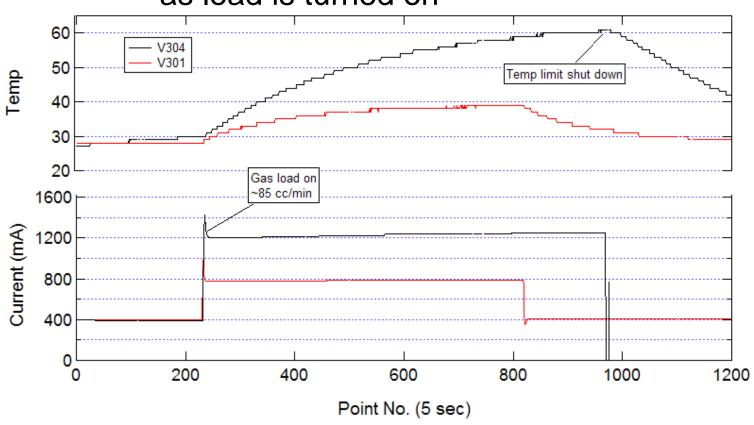
V304 ultimately shut down due to 60C temperature limit
