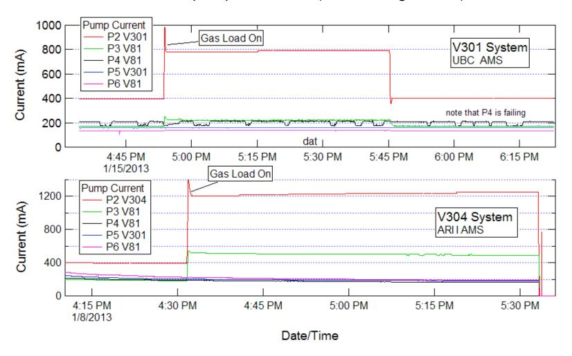
V304 running at 50% higher load than V301. P3 also running ~50% higher.
