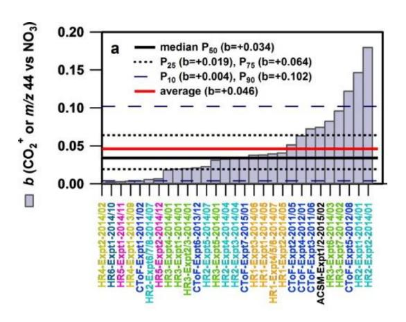
Pieber Effect: Charred OA residue on the vaporizer reacting with nitrate salts to form excess CO<sub>2</sub><sup>+</sup>
