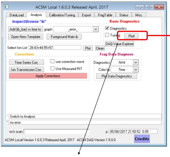
Can also use DAQ Value Explorer to plot time series of the other ~80 housekeeping parameters recorded by DAQ
