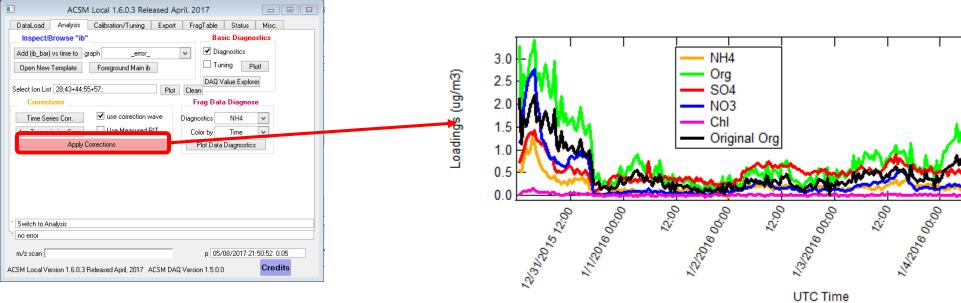
Time series correction can have a big effect on calculated mass loadings
