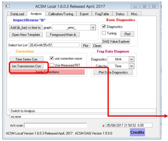
Relative Ion Transmission: Correct for poor transmission of larger m/z ions through the quadrupole.
