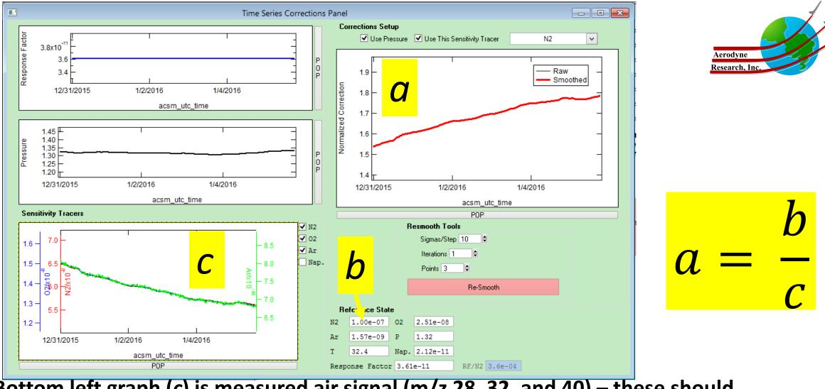
Bottom left graph (c) is measured air signal (m/z 28, 32, and 40) – these should do the same thing
