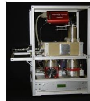
ACSM with the Pfeiffer pumps and integrated power supply S/N: 140-110 Feb 2011
