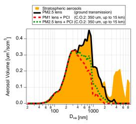
Current PCI with large C.O.2 can achieve better E<sub>L</sub> than PM1 lens at ~15 km alt.
