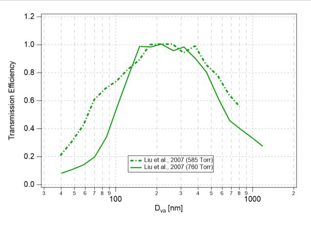
PM1 curve is slightly better at lower ambient pressure (Liu et al., 2007)
