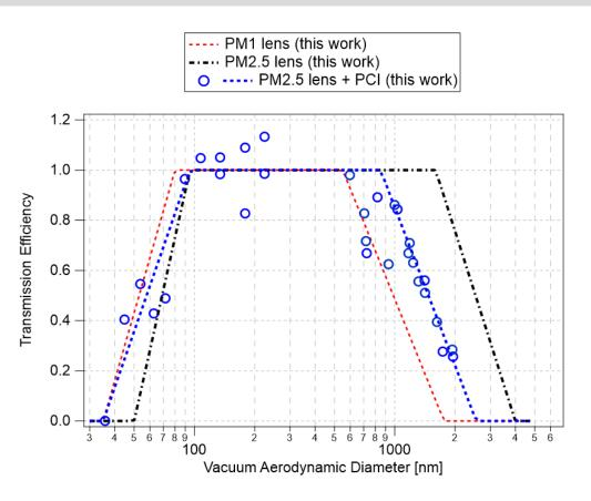
Coupling with PCI worsen the transmission in the high end but still better than PM1 lens but slightly improve the low end.
