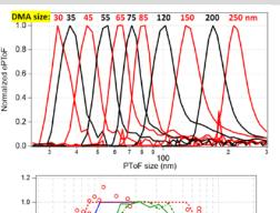
Can generate monodisperse aerosols (30-300 nm) without doubly charged particles.
