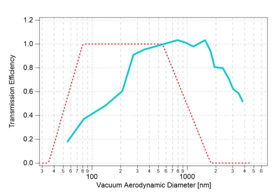
Xu et al. reported E<sub>L</sub> curve for the new PM<sub>2.5</sub> lens showing much better transmission for large particles but much less transmission for small particles.
