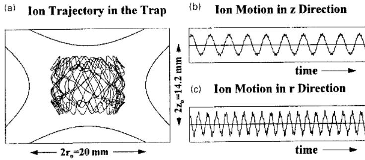
**Figure 13-24** Simulation of motion of a single trapped ion in an ion trap: (a) shows the overall motion within the trap in cross section, (b) shows the time-dependent component of motion in the axial direction, and (c) shows the radial-direction component.
