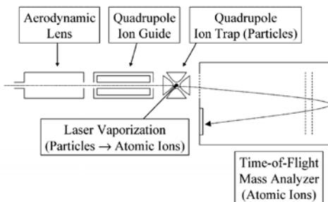
**Figure 1.** Basic design of the nanoaerosol mass spectrometer.
