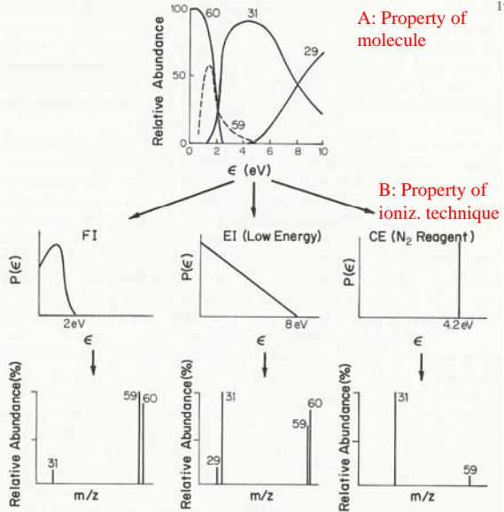
**Figure 14-29** Convolution of the breakdown curve (top, an intrinsic property) with the internal energy distribution ( $P(\epsilon)$ ) resulting from different ionization techniques under particular experimental conditions to produce mass spectra of 1-propanol. FI indicates field ionization, a soft ionization method used for vapor phase samples.
