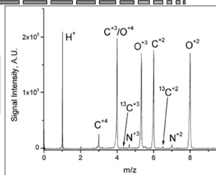
**Figure 2.** Low  $m/z$  region of the mass spectrum of  $\sim$ 10-nm-diameter sucrose particles, average of 50 individual spectra.
