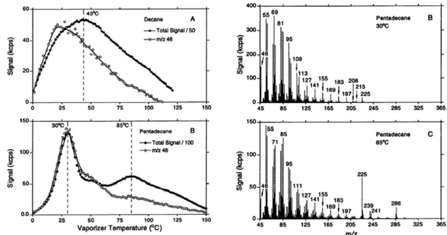
FIGURE 3. Thermal desorption profiles of SOA formed from reactions of (A) decane and (B) pentadecane with OH radicals in the presence of  $\text{NO}_x$ . Total signal was divided by the factor shown in the legend.
