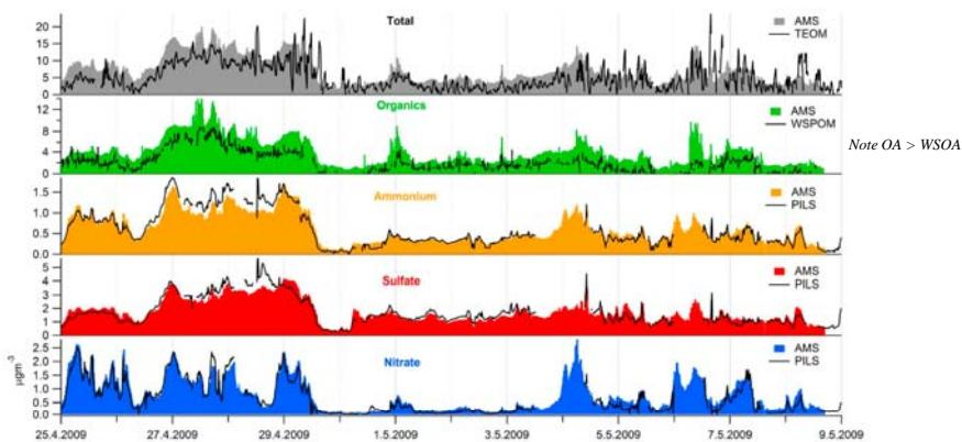
**Fig. 2.** Concentrations of major ions and WSPOM (using conversion factor 1.6 to convert WSOC to WSPOM) measured by PILS-TOC-IC and AMS from 25 April to 8 May 2009. PILS-TOC-IC (ions, WSPOM) and TEOM (total mass) results are marked with the black line. AMS results are marked with colors (blue = nitrate, red = sulfate, yellow = ammonium, green = total organics, grey = total mass i.e. sum of ions and organics).
