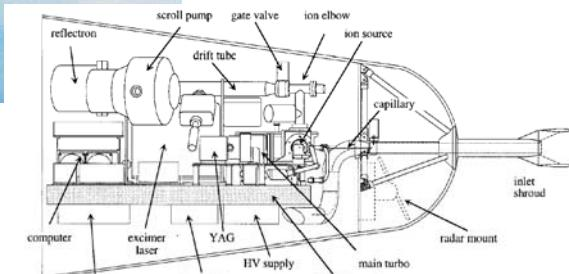
FIGURE 3. Schematic layout of the PALMS instrument components. For scale, the carbon fiber table is 122 cm (48") long.
