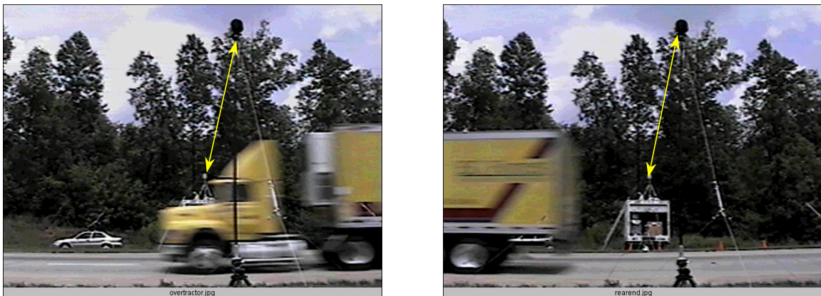
Figure 7-6: Two video frames taken during an emission measurement on I-40
