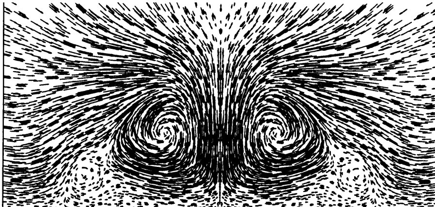
Figure 4-3: Computed speed vectors at a cross section normal to the vehicle velocity at \frac{1}{4} car lengths behind the automobile (Johnson et al., 1996)
