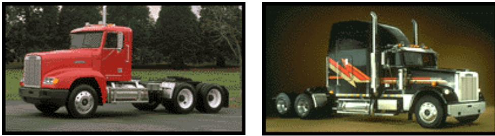
Figure 7-1: Two heavy-duty truck tractors showing the location of the exhaust pipes
