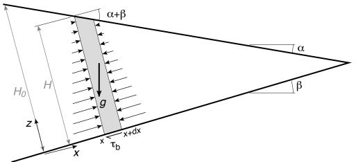
Consider the force balance in the x direction on the shaded region of width dx. Note that gravity will have a component of force in the negative x direction. We find when we balance this that
