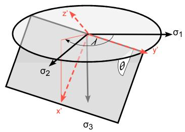
Consider a case where  $\sigma_1$  and  $\sigma_2$  to lie in the horizontal plane and we wish to know the slip resolved onto a plane with a dip of  $\theta$  and a dip direction of  $\lambda$  measured from the x ( $\sigma_1$ )-axis
