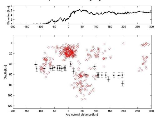
South (left) to north (right) cross section of topography (black solid line), seismicity (red circles) and crustal thickness (black bars) across the Himalaya of Nepal and Tibet. Earthquakes cluster in the midcrust beneath the region of maximum relief along the Himalayan front, a zone also identified as a locked zone from GPS measurements.
