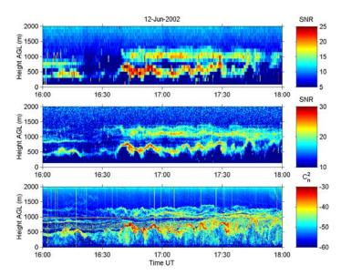
The range resolution of the data shown in the upper panel of the figure is 105-m. The same data have been RIM processed and are shown in the middle panel. It is clear that much more atmospheric structure has been revealed using the RIM technique. The FMCW radar data shown in the lower panel confirms this. Although not shown here, RIM can also be used to obtain wind estimates at high vertical resolution.
