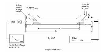
Experimental layout of the Cavity Ring Down System
