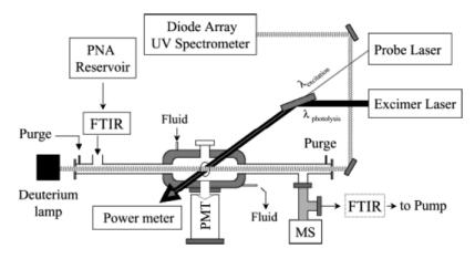
Schematic of the experimental apparatus used to measure the rate coefficients for the reaction of peroxynitric acid and hydroxyl radical.
