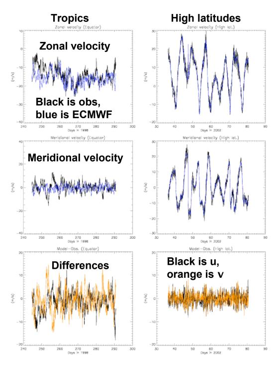
Comparison of direct wind measurements with ECMWF analysed winds in long-duration stratospheric balloon flights (at 60 hPa) leads to the same conclusion
