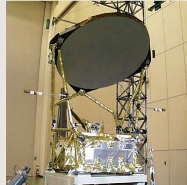
photo: AMSR-E instrument (160 cm aperture, 7 Ch) 120-cm GPM-GMI also conical)
