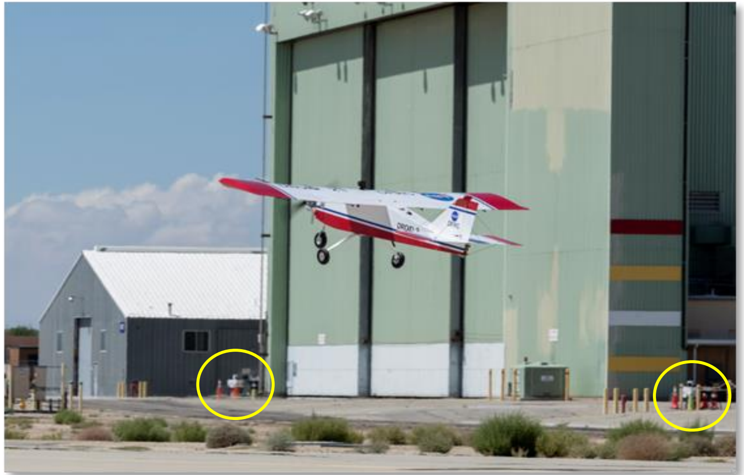
2023 lidar installation at AFRC Lidars were set for 24/7 automated operation
