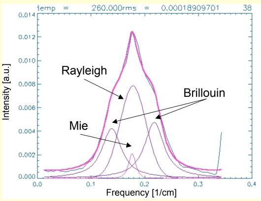
Spectral measurement deconvolved and separated into Mie, Rayleigh, and Brillouin components
