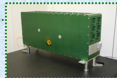
DAWN Transceiver (Transmitter + Receiver) 250 mJ/pulse, 10 pulses/sec. 5.9" x 11.6" x 26.5", 75 lbs.; 15 x 29 x 67 cm, 34 kg (no telescope or scanner)
