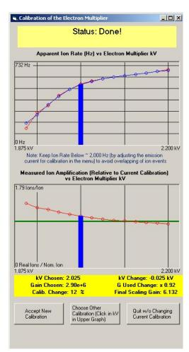
• Once the curve 'plateaus,' the increase in signal with gain is maximized and a further increase in voltage will not increase the signal but will shorten the lifetime of the multiplier.
