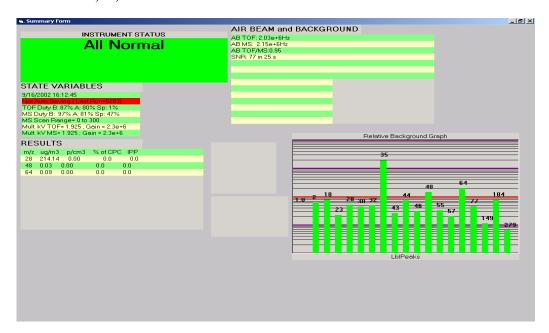
Note: The relative background graph shows the ratio between the current background values for some of the background peaks and a typical reference background for an AMS instrument (The current reference used comes from the CalTech Aircraft AMS).
