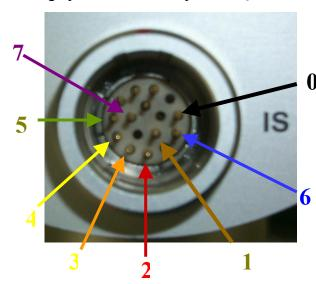
QMS pin diagram. Voltages should be measured relative to the ion reference to get actual voltage values (i.e., if extraction is 150 V, should get 150 V measuring between ion reference and extraction pins.
