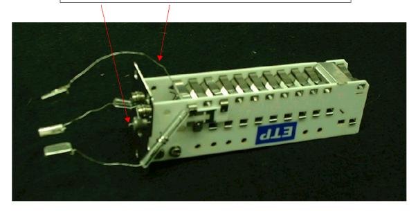
Note: If the replacement multiplier has a protective metal coverplate make sure that it is removed!
