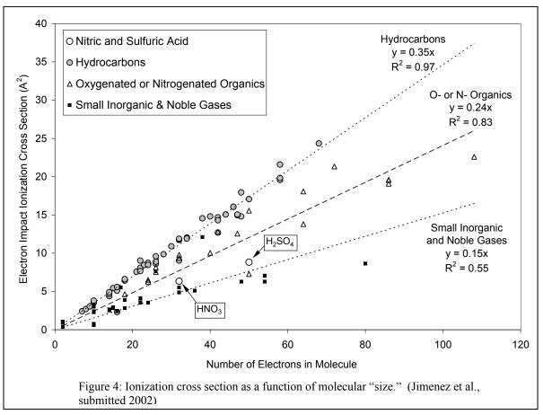
Figure 4 shows that for small molecules of a given type,  $\sigma/N_e$  is approximately constant. From the data and regressions in the figure  $R_t$  is estimated at 0.57 for hydrocarbons, 0.83 for oxygenated hydrocarbons, and 1.12 for sulfuric acid. Experimental verification of this relative calibration procedure with individual aerosol molecules is undergoing in our laboratory and will be the subject of a future publication.
