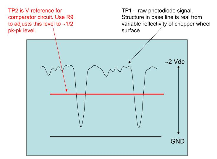
Raw chopper photodiode signal is "cleaned" using an opamp/comparator. TP1 and TP2 are the inputs to the comparator. The output of the comparator is the chopper signal that the computer monitors.
