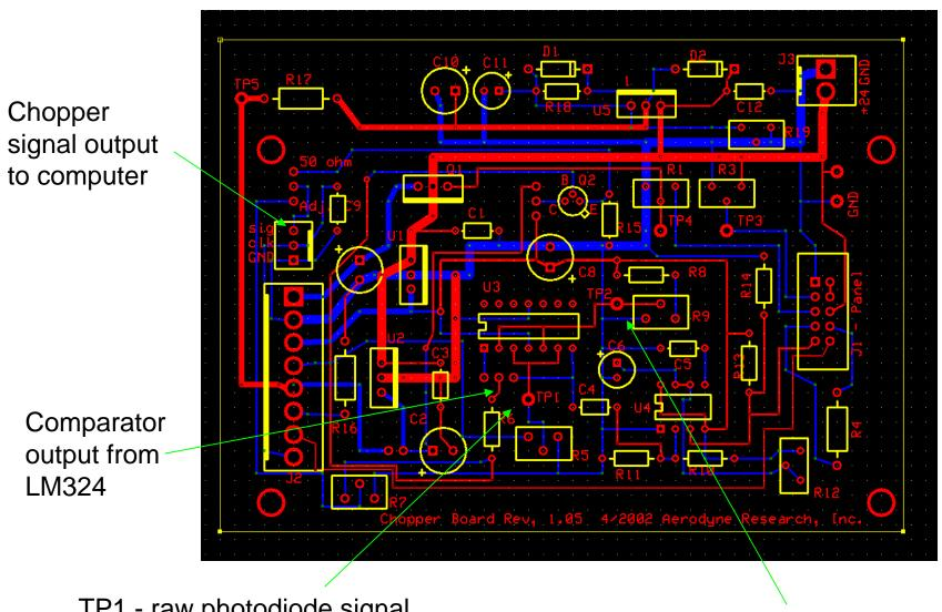
TP1 - raw photodiode signal
