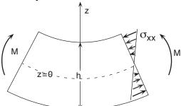
First, consider the stresses acting on the edge of the plate (these are deviatoric stresses; we have subtracted out the mean stress P/h). The total moment is
