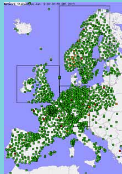
The present European network of GNSS stations used in weather forecasting. Courtesy of the E-GVAP programme (link on p. 31) of short, medium or seasonal term water vapour distribution on a global scale. The left-hand figure gives such an example.
