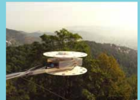
A GNSS installation for vegetation and soil moisture measurements. Courtesy of A. Egido, Starlab
