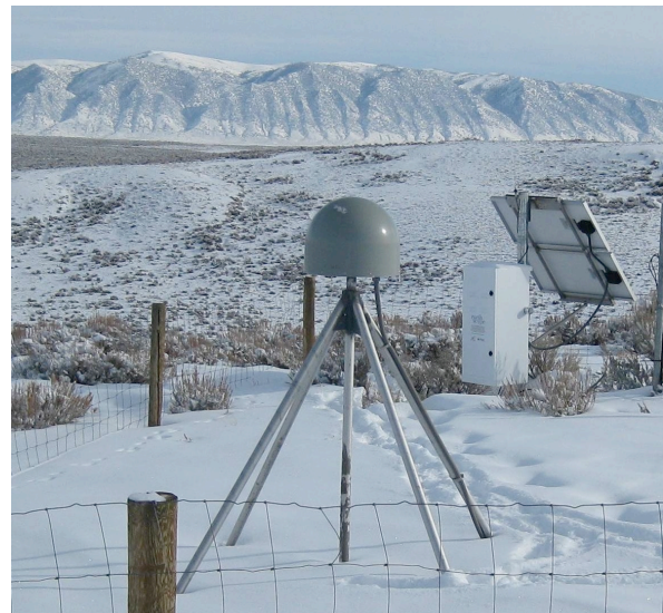
Figure 1. Geodetic-quality GPS site located near Randolph, Utah. It is operated by UNAVCO for the EarthScope Plate Boundary Observatory. Solar panels and batteries are used to power the GPS receiver, which is stored in the white equipment box shown in the background.
