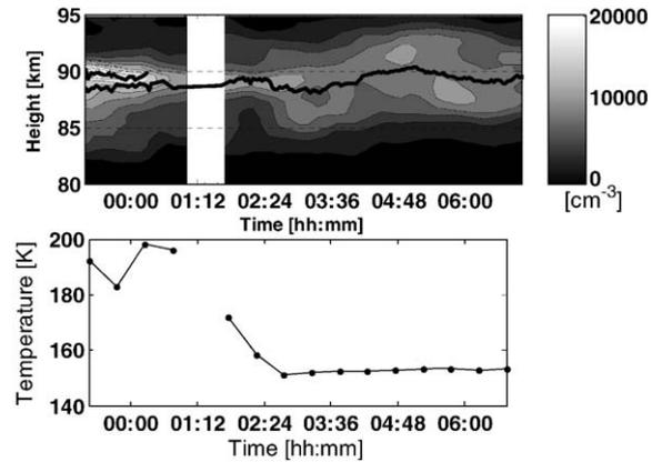
Fig. 6. (top plot) A contour plot of the iron density with calculated layer height of Fe (black line) and  $\text{Fe}_S$  (dashed black line) for the 28 January, 2003, from 23:10 to 07:25 UT. (bottom plot) The corresponding mean temperature calculated between 85 and 95 km for every half hour. See text for more explanation.
