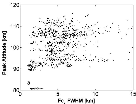
Fig. 3. Peak altitude versus FWHM of sporadic Fe layers at Rothera. Each dot represents one lidar profile of 2.5 min integration time.
