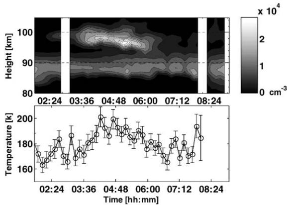
Fig. 7. (Top plot) shows a contour plot of the iron density for 25 February, 2003, from 02:30 to 07:30 UT. (bottom plot) shows the corresponding mesospheric hydroxyl temperature measured with the Bomem spectrometer located at Rothera.
