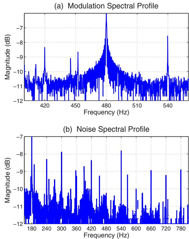
**Fig. 4** Autocorrelated Fourier spectrum for the modulation spectral profile showing the (a) degree of spectral broadening and (b) noise spectral profile centered about the 480-Hz modulation frequency. Note the 60-Hz harmonics and noise components about 450 Hz (a). Also note the extensive noise throughout and the 60-Hz harmonics (b). These results may not be universal, but may serve as an example.
