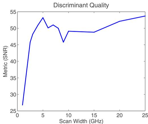
**Fig. 6** A plot of the discriminant SNR versus scan width; modulation amplitude and scanning ramp voltages were scaled to compensate for the changing scan width in order to isolate the dye-ring-laser control box as a source of noise.
