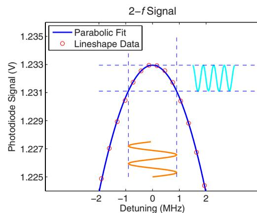
**Fig. 10** A graphic showing the Doppler-free Na  $D_{2a}$  absorption peak with a modulation added to model the  $2-f$  response signal; note that this places an upper bound of  $\sim 1$  MHz on the modulation's amplitude.
