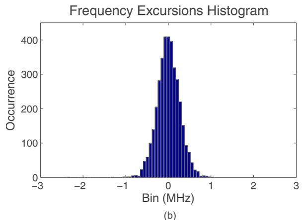
**Fig. 7** (a) Excursions from the center frequency recorded at 1-s intervals and (b) a histogram generated from the same data. Wavelength meter temperature drift was removed by subtracting a 20-s sliding/boxcar average.
