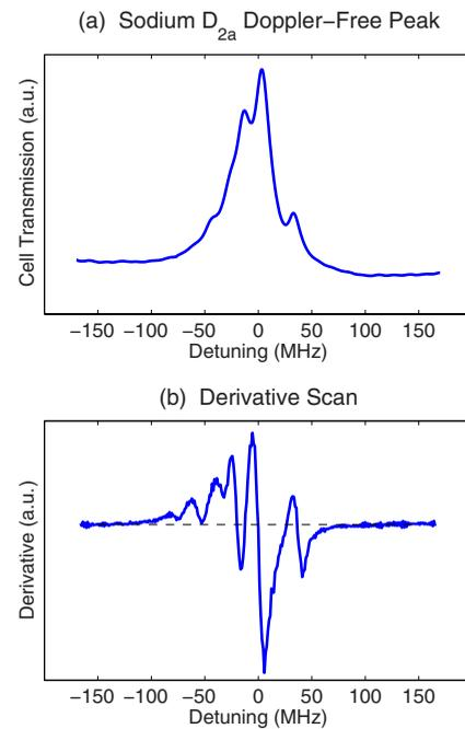
**Fig. 2** (a) Recorded Doppler-free spectrum at the Na  $D_{2a}$  absorption line and (b) the derivative signal obtained from wavelength modulation.
