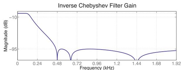
**Fig. 5** An inverse Chebyshev filter with 95-dB stopband attenuation and 120-Hz passband implemented in the phase sensitive servo loop; note the stopband nulls at  $1-f$  (480-Hz) and  $3-f$  (1440-Hz) harmonics; cutoff and sampling frequencies are 465 and 5750 Hz, respectively.
