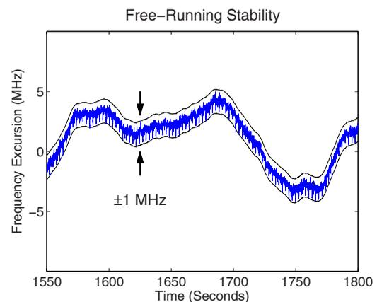
**Fig. 3** Time series of wavelength meter-recorded frequency excursions from the mean showing the free-running stability of the dye ring laser; the laser control box was set to "lock" (internal servos engaged).
