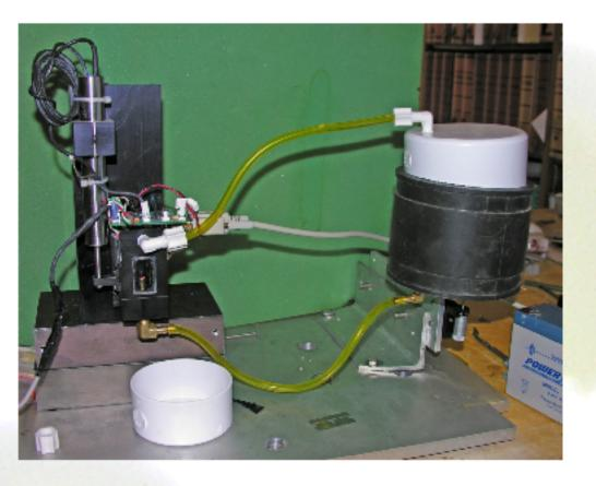
In the pilot design we found that the motor actuator had too much inertia to respond to meniscus fluctuations sufficiently rapidly, and overshot the equilibrium point resulting in "hunting". The system is now being re-designed around a woofer speaker coil that will respond to 1000 times faster.
