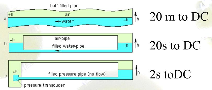
No flow occurs in (c) but the pressure sensor tends to drift and to require frequent calibration to detect reliablysmall pressures (<5 mm of water height). We have tested a new meniscus pressure sensor that overcomes this propensity to drift by using a servo-controlled orifice whose elevation is shifted to null pressure changes caused by tilt.
