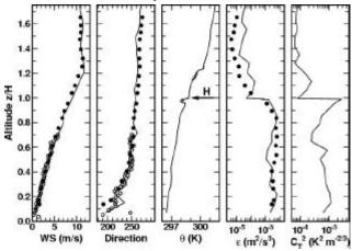
Comparison plots of TLS data (solid lines), minisodar data (open circles), and Doppler lidar data (solid circles) from the Pentagon Shield experiment in Washington, DC. Data were obtained using a preliminary version of the improved TP, demonstrating the utility of the TLS system for in-situ verification of remote sensing data
