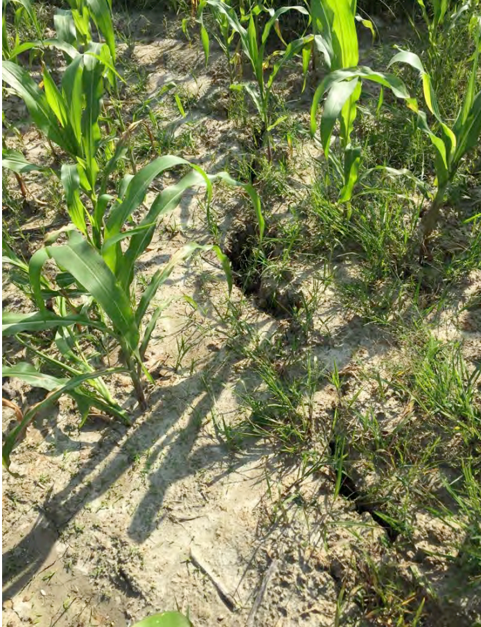
Figure 5 (left): Liquefaction crack with silt covering soil layer.
