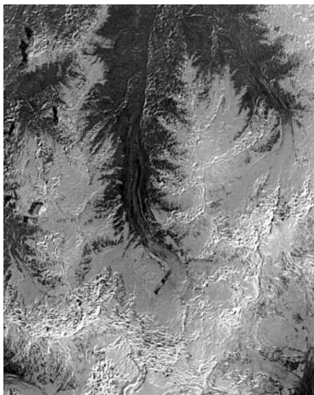
Fig. 5. SPOT 3 spectral band 3 image of the Raikot basin after topographic normalization using the Lambertian assumption. Much of the reflectance variability found in the original image (Fig. 4) has been reduced, although image artifacts are present as a result of overcorrection.
